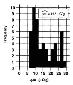
Figure 4. Frequency distribution of toner particles as a function of q/m.
