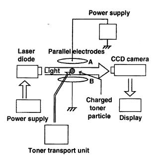
Figure 1. Schematic configuration of a technique for measuring q/m.
