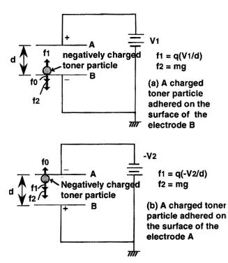
Figure 3. Detailed schematic expression of the parallel electrodes.
