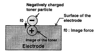
Figure 2. A charged toner particle adhered on the surface of the electrode.
